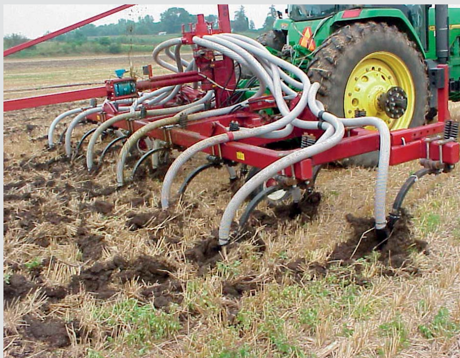
Manure injection into wheat stubble. (Photo credit: Charles Gould)
